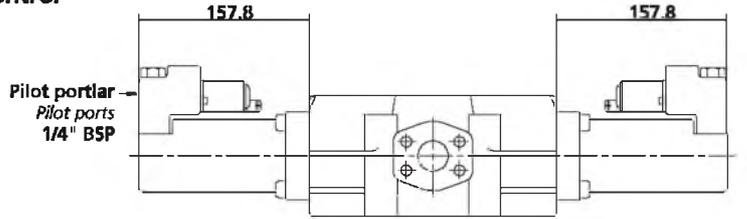
**PILOT VALFLER & PILOT UYGULAMA VALFİ / PILOT VALVES & PILOT SUPPLY VALVE****HPV/HPVL PİLOT VALFLERİ / PILOT VALVES HPV/HPVL**
